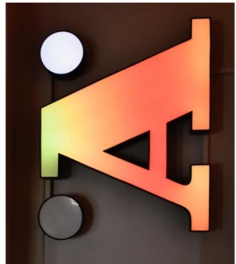
an old signage "Ä", visualizing weather with color LEDs, controlled by a P44-LC
